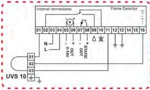
Make a good connection of the ground of AF1 to the body burner ground to ensure correct operation.
