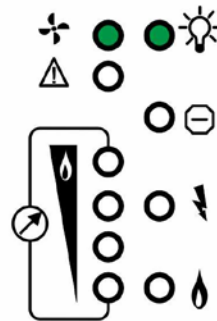
Power Supply + enabled
