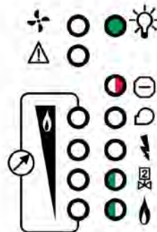
Ev1 Gas Not Connected Block
