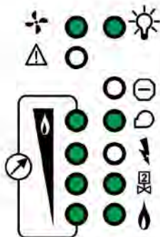
Flame Detect Flame Signal Ev1 Gas Ev2 Gas
